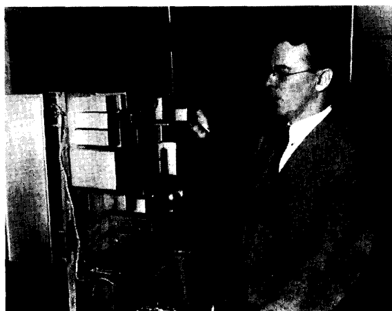
Harold S. Black in 1941 with some of the amplifying equipment that used his idea for reducing distortion by reversing some of the amplifier's output and feeding it back into the input. (Photo: AT&T Archives)
